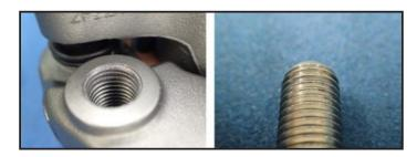
If the threads are stripped or otherwise damaged, the caliper must be replaced. Use an Online Tech Request to submit a photo of the damage before proceeding. Follow Ténéré 700 Service Manual (P/N: LIT-11616-35-55) procedures to replace the caliper and union bolt gaskets. Bleed the brake system using Yamalube DOT 4 Brake Fluid (P/N: ACC-BRAKE-FL-UD).
