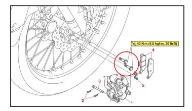
3. If either bolt or both bolts are incorrect, clean the mounting hole threads in the caliper. Visually inspect the threads for damage and use a clean bolt of the correct type to see if it can be threaded into the hole smoothly.
