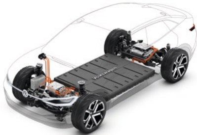
All the cars in the ID. family are based on the new MEB platform (modular electric drive matrix).
