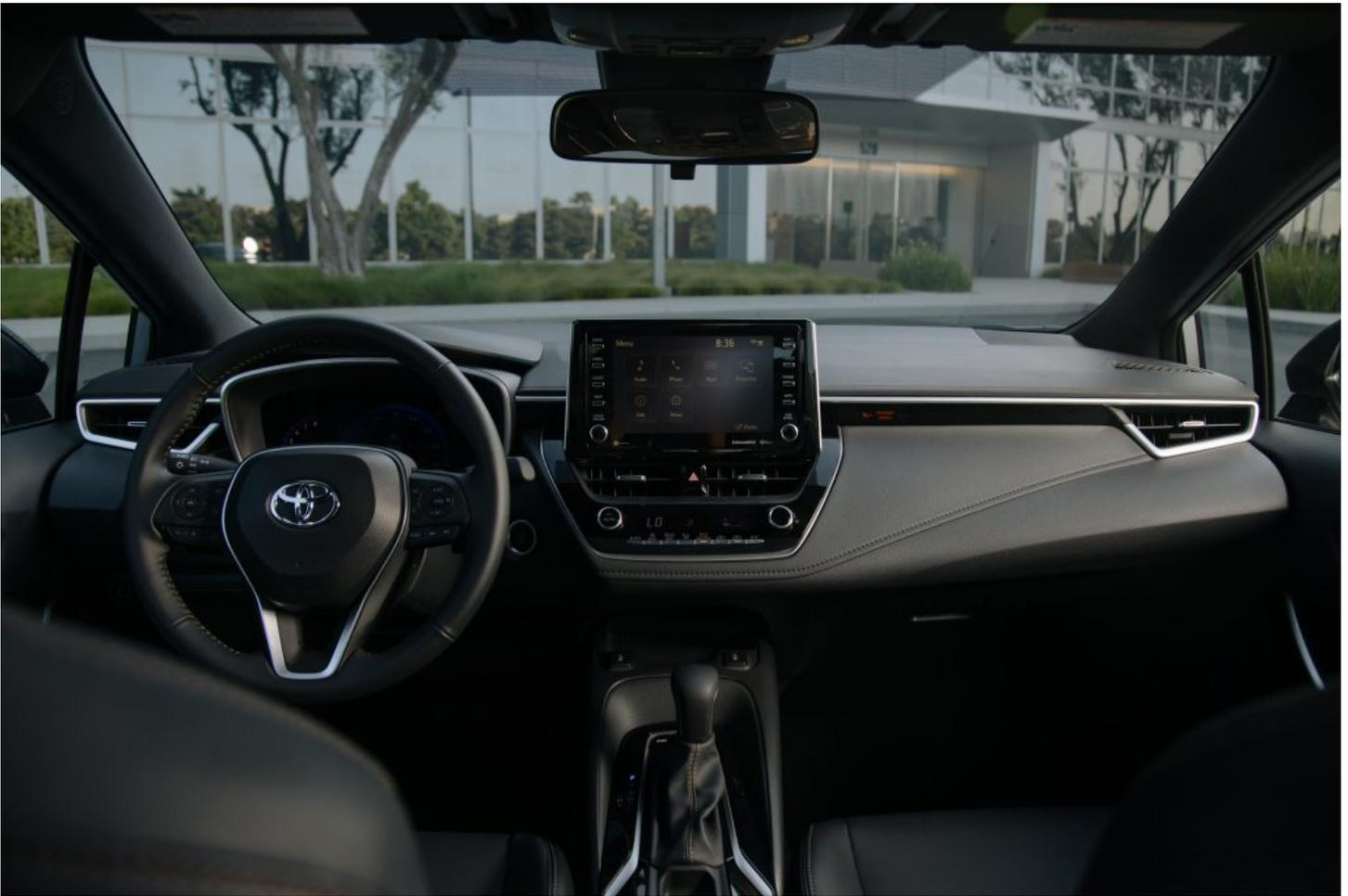
The standard audio multimedia system on both the SE and XSE grades includes an 8-in. touch-screen display; six speakers; Android Auto™ & Apple CarPlay® & Amazon Alexa compatible, USB media port, 1 USB charge port, hands-free phone capability and music streaming via Bluetooth® wireless technology, and SiriusXM® with 3-month All Access trial.
