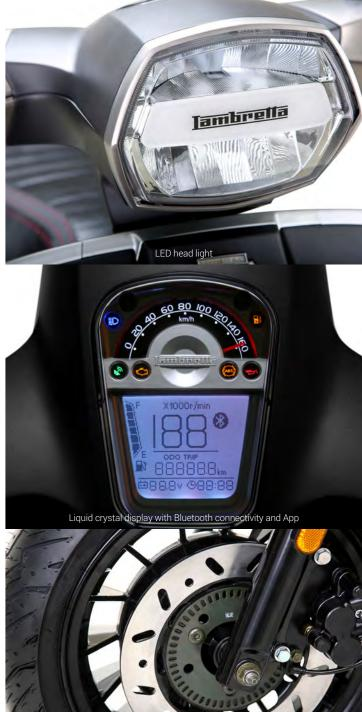
Front and rear disc break (V200 Special with Bosch ABS System)
