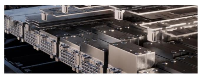
Boasting a large capacity 111kW battery (107kW usable), the Volvo EX90 brings a new dimension to all-electric driving for the brand. The 17 modules are arranged within the floor of the vehicle and the configuration lowers the centre of gravity of the car and has the additional benefit of allowing for enhanced interior space thanks to a completely flat base.
