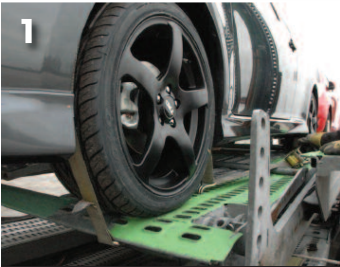
Photo 1: Correct Wheel Straps
