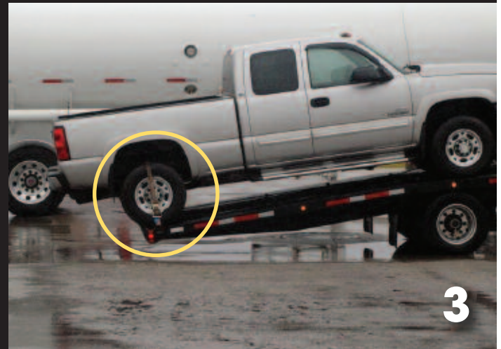
Photos 2 and 3: Incorrect Wheel Straps
