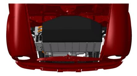
Swindon Powertrain also offers a range of optional components including a purpose designed 12 kWhr battery pack, which fits under the original bonnet in place of the internal combustion engine, motor controller, onboard charger and DC-DC converter, speed sensor kit and cooling system pump, with orders books for these additional items also open.
