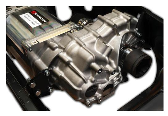
The Classic Mini Kit package comprises an HPD E Powertrain system mounted to an original classic Mini front subframe featuring brackets specifically designed for this installation. It also includes purpose designed inner CV joint housings that allow the fitment of standard Mini driveshaft assemblies and comes complete a standard differential (optional limited slip differential available).
