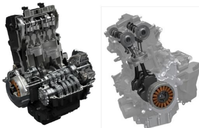
776cc, four-stroke, liquid-cooled, DOHC, parallel twin engine
