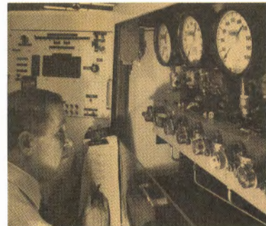
Automatic Solenoid Test Console - Several operational tests are automatically performed on as many as eight solenoids in one test cycle.
