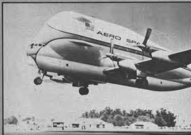
The second Aero Spacelines creation, called the "Super Guppy." This particular machine used the wings and engines from one of the YC-97Js based at Norton AFB near San Bernardino. The first flight of the Super Guppy took place on 31 August 1965.
