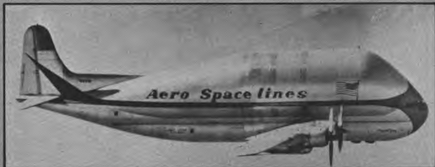
The "Pregnant Guppy," a standard Boeing 377 stretched and fitted with a new fuselage which more than doubled its original volume. The entire tail is unbolted and rolled away in order to load over-
