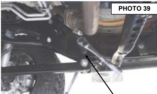
Tighten the lower drop hardware.
