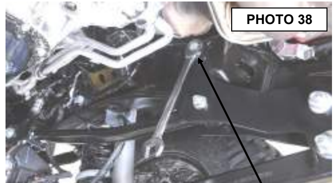
Tighten the upper drop hardware.
