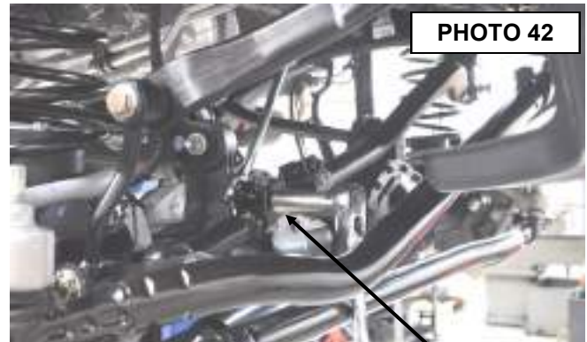
Adjust forged track bar.
