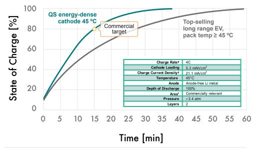
†C/3 (1.76 mA/cm2) used from 0-10% SOC, 4C (21.1 mA/cm2) used from 10% to upper cut-off voltage (4.25V) ‡Commercially relevant dimensions may vary from 60x75 mm to 70x85 mm, depending on cell format
