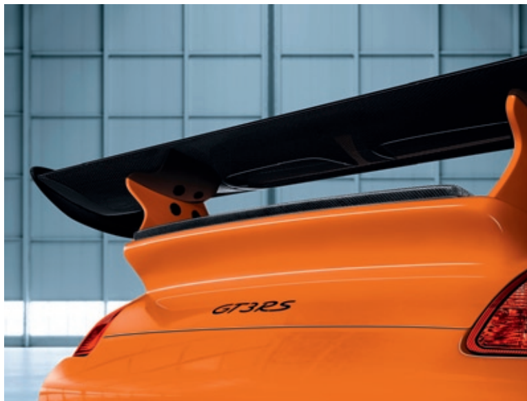
Spoiler lip on rear wing in carbon (Gurney Flap)
