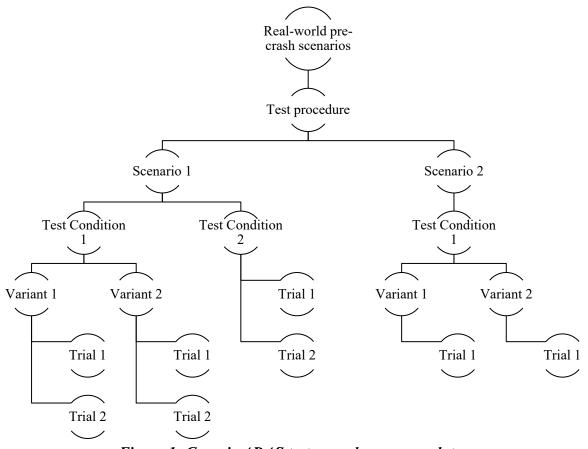
Figure 1: Generic ADAS test procedure nomenclature
