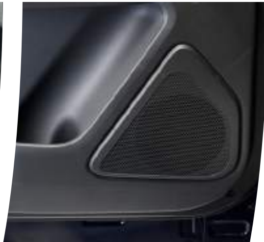
6 speaker system with carbon nanotube speakers
