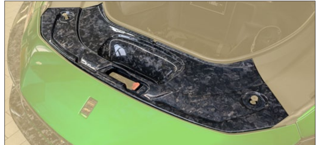
Trunk cover visible carbon fibre primed without clear coat
