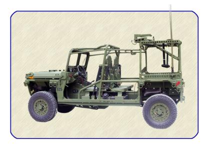
GROWLER manufactures the M1161 Light Strike Vehicle (LSV) and M1163 Prime Mover (PM). These vehicles are used by the United States Marine Corps Special Operations Command (USSOCOM), and fielded as a light attack vehicles to support expeditionary forces. The M1161 and M1163 are the only production tactical vehicles certified by the US Military to fly in the V-22. Our design includes a hinged pintle hook, removable and collapsible roll cage and vehicle stacking capability.
