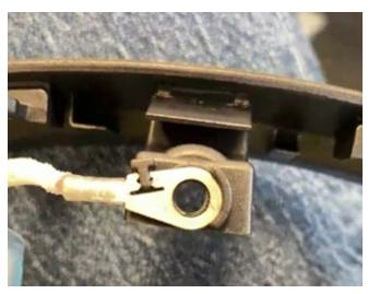
Note: DO NOT check the cable lug of the ground strap for tightness.
