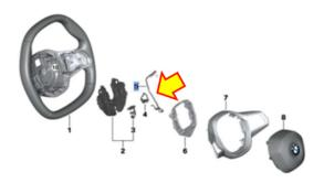
Remove the steering wheel airbag. Check the ground wire at the steering wheel horn pad bracket for correct tightness and lack of movement.
