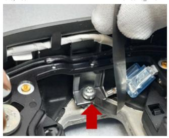
5. If there is no relative movement, use a 0.1 mm feeler gauge between the bottom of the screw head and the horn pad bracket.
