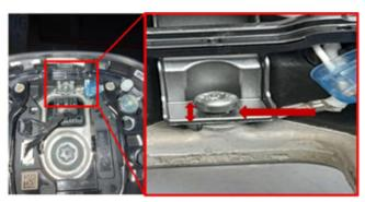
3. If the ground connection screw is not in contact with the horn plate bracket upon visual inspection but is tight and at the correct torque spec (2.5 Nm +- 5 Nm), the screw must be removed, and the threads need to be inspected for any burr formations.
