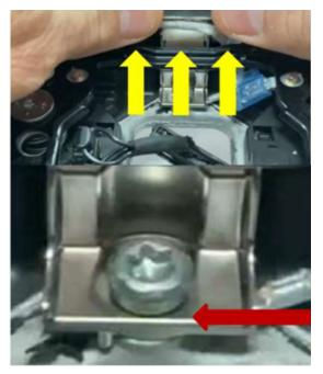
Press the horn cover from the inside out to observe any possible movement of the horn pad bracket and the screw.
