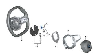
2. Remove the steering wheel airbag following the repair instructions listed in ISTA/AIR 32 34 030 and check the ground connection.
