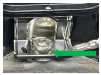
4. If the screw is already in full contact with the horn plate bracket and is tighten to (2.5 Nm + - 5 Nm), check the tightness of the connection as explained below.
