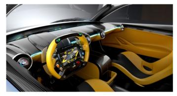
Above the dashboard, an under-windshield eyelid integrates the three displays that offer views to the rear and sides of the car. Here too, the wing mirrors have been replaced by cameras. Their placement is designed to have the rear view immediately after the front view, without moving one's head.
