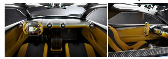
The wing-shaped, horizontal sports dashboard has a dark, carbon-printed leather upper part and a yellow sports leather lower part, separated by a chrome strip that integrates the four individually adjustable air vents.
