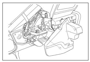
After you have completed the inspection procedure, apply a second punch mark on the right frame spar, just above the rear master cylinder reservoir as shown.
