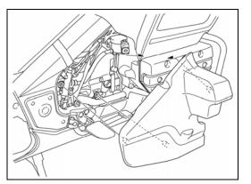
Look for a punch mark(s) on the right frame spar, just above the rear master cylinder reservoir as shown.
