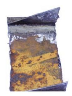
surface that prevents rust. I put a section of tunnel from a 68 VW floorpan into this solution to soak for several hours but the results weren't that encouraging, especially given that it would be practically impossible to dip an entire floorpan. On bar and sheet metal, however, it worked really well, and did everything that it claimed.
