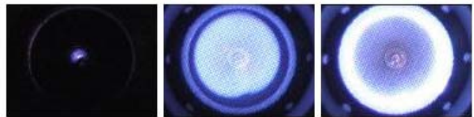
Figure 15. Combustion Sequence for Std. Ignition \Phi = 0.770 (Lean Limit), 16 ms per Frame
