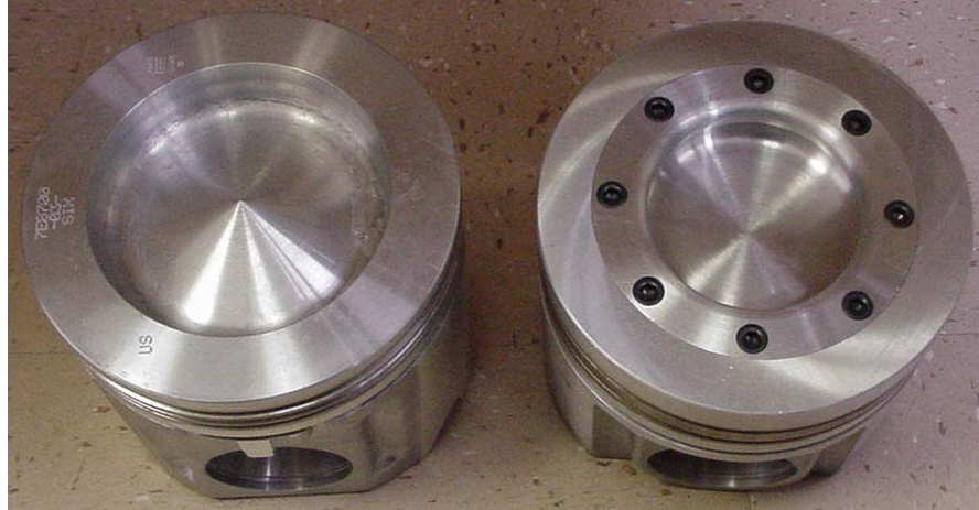
Figure 6. Diesel Piston (Left) was Modified (Right) to Accept RFEIS
