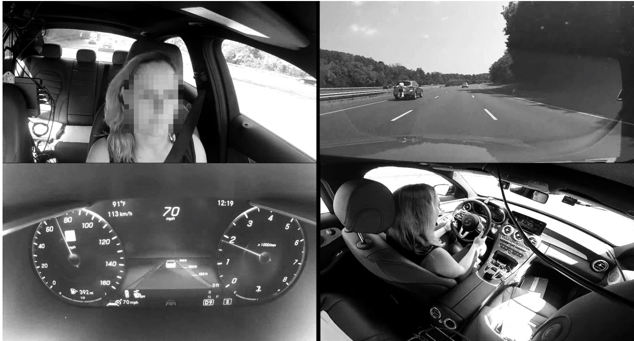
Figure 1. Still frames depicting the camera angles used to capture the driver's face, forward roadway, instrument cluster, and front seats. Top right frame shows the bear vehicle during a reveal from the participant's point of view.
