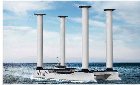
3/4 front view of the FARWIND energy ship with rotor sails ©Cabinet
