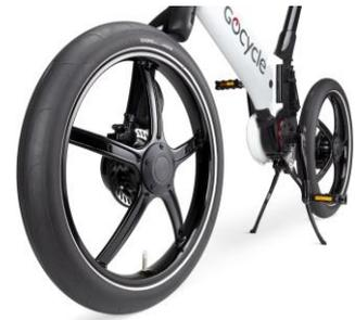
The Gocycle G4's removeable powerful Lithium-Ion battery is seamlessly integrated into the G4's hydroformed aluminium frame. It provides a range of up to 40 miles (65km) for the G4 and up to 50 miles (80km) for the G4i (depending on pedal input) with 3.5 hour fast charging now standard across the entire range from Gocycle's new 4A 36V Charger.
