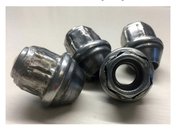
7. In the picture below, it is apparent that the lug wrench supplied to Plaintiff Desotelle by Ford is completely useless as it does not fit on the swollen and delaminated lug nuts, which rendered it impossible for Mr. Desotelle to remove and replace his wheel when he got a flat tire.
