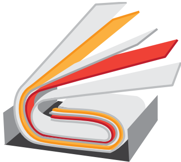
Conventional Wound Lithium-ion Cell
