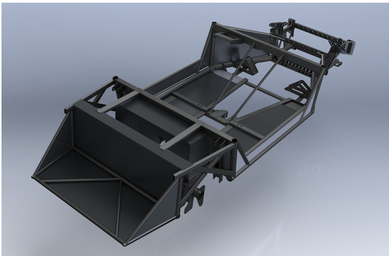
View telaio3 / 4 rear panels positioned aluminum honeycomb
