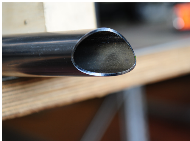
Tubular component of the frame automatically cut with laser
