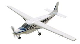
**Oshkosh, WI (July 25, 2022)** Ampaire today announced a key exclusive supplier for the hybrid-electric propulsion system it is developing for its Eco Caravan aircraft, an upgrade to the current Cessna Grand Caravan. Ampaire will use a RED Aircraft AO3 series compression ignition engine rated to 550 hp (405 kW) in an integrated parallel configuration. The RED engine provides the base power and the Ampaire electrical system provides the peak power.
