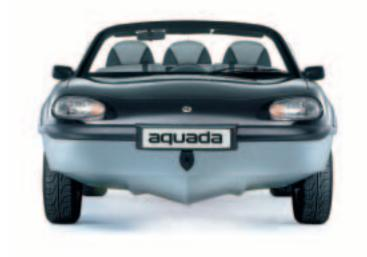
A RADICAL NEW BREED This vehicle is made possible by the application of High Speed Amphibian (HSA) Technology. Its ability to 'plane' on water is the result of a 7 year development programme and engineering breakthroughs culminating in over 60 patented inventions. These include a revolutionary jet propulsion system that delivers nearly a tonne of thrust, computer controlled wheel retraction and leading edge developments in hydrodynamics.
