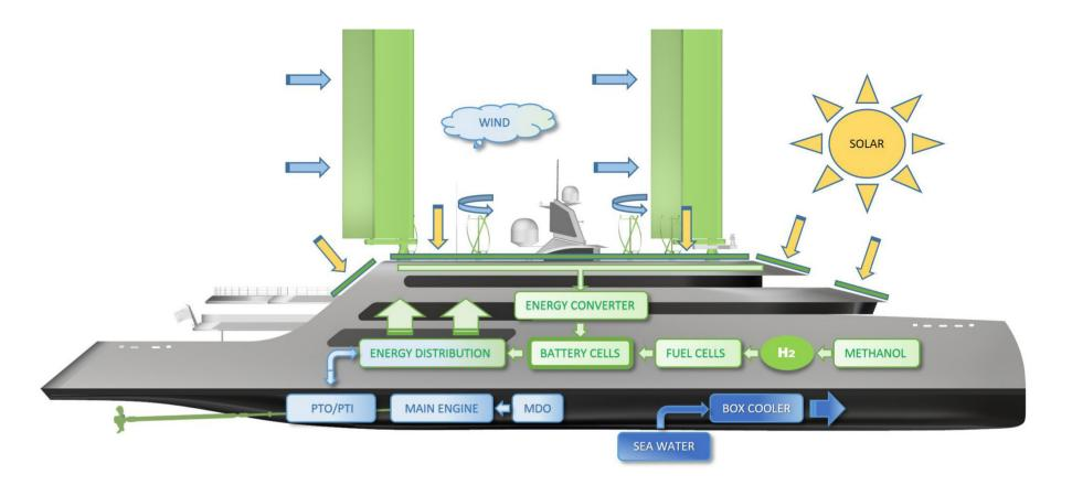
Utilising 6 box coolers instead of a conventional pumped cooling system, main engines, air conditioning machinery, fuel cells and other equipment become more efficient due to the reduction of electrically driven pumps required. This has the possibility of saving approximately 70kW of electrical power per hour.
