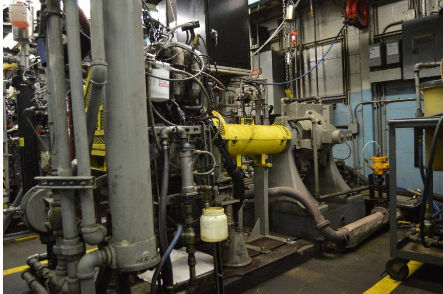
Figure 6: Ford 2.3L fuel quality research engine on dynamometer Image Source: AAA
