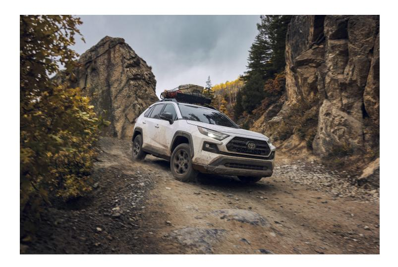
For maximum capability and prowess on the trails, there are the Adventure and TRD Off-Road grades. These models come with Dynamic Torque Vectoring AWD with Rear Driveline Disconnect standard. In addition to directing up to 50 percent of engine torque to the rear wheels, this system can also direct more torque to the left or right rear wheel to enhance on- or off-pavement handling.
