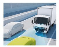
3) Lane Keep Assist < First introduction in a Japanese light-duty truck\*3 > Recognizes right and left lines of a cruising lane with integrated cameras, electrically assists and controls the steering wheel handling to help lane keeping and prevent lane departure, contributing to reducing driver fatigue and enhancing safe driving.
