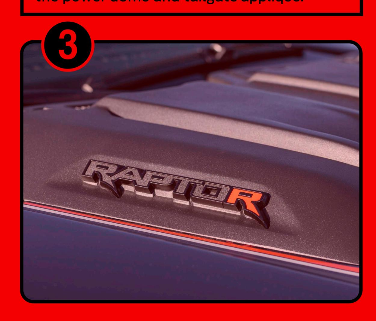
**EXTREME STYLING:** A taller, more aggressively styled power dome on the hood highlights the supercharged V8 engine underneath. It sits nearly one inch taller than on the base Raptor, helping extract warm air from underneath.
