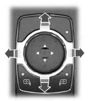
To adjust your mirrors, switch your vehicle on, with the ignition in accessory mode or the engine running.
