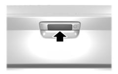
Pull up on the handle to release the tailgate.
