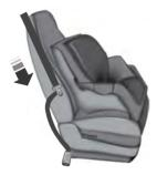
After positioning the child restraint in the proper seating position, pull down on the shoulder belt and then grasp the shoulder belt and lap belt together behind the belt tongue.
