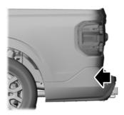
The sensors are behind the rear bumper on both sides of your vehicle.
