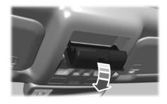
The glasses holder is in the overhead console. Press near the rear edge of the door to open.
