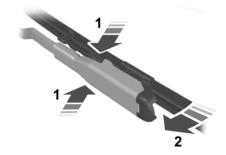
Lift the wiper arm and then press the wiper blade locking buttons together.
