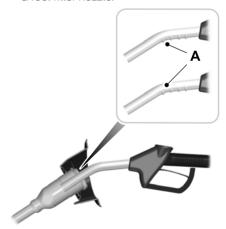
Insert the fuel pump nozzle up to the first notch on the nozzle A. Keep it resting on the cover of the fuel tank filler pipe opening.
