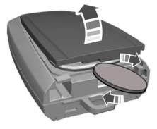
2. Twist a thin coin under the tab hidden behind the key blade head to remove the battery cover.
