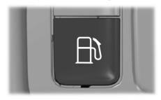
Press the button on the left side of the instrument panel next to the headlamp switch to open the fuel filler door. The fuel filler door can take up to 15 seconds to open before you can insert a fuel filler nozzle.
