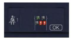
This warning displays if an occupant unfastens the rear seatbelt buckle or it becomes unfastened.
