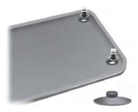
To install floor mats that have eyelets, position the floor mat eyelet over the retention post and press down to lock in position. Repeat for all eyelets on the floor mat.
