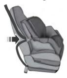
While holding the shoulder and lap belt portions together, route the tongue through the child restraint according to the child restraint manufacturer's instructions. Make sure that you did not twist the belt webbing.
