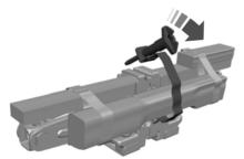
2. Remove the jack and tool bag from the jack bracket.
