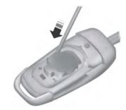
4. Insert a screwdriver as shown to release the battery.
