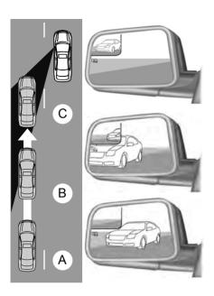
The image of the approaching vehicle is small and near the inboard edge of the main mirror when it is at a distance. The image becomes larger and begins to move outboard across the main mirror as the vehicle approaches (A). The image transitions from the main mirror and begins to appear in the blind spot mirror as the vehicle approaches (B). The vehicle transitions to your peripheral field of view as it leaves the blind spot mirror (C).
