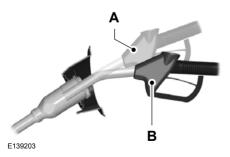
4. Hold the fuel pump nozzle in position B when refueling. Holding the fuel pump nozzle in position A can affect the flow of fuel and shut off the fuel pump nozzle before the fuel tank is full.
