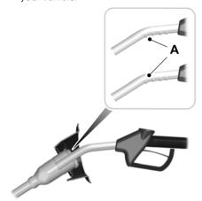
Insert the fuel pump nozzle up to the first notch on the nozzle A. Keep the fuel pump nozzle resting on the fuel tank filler pipe.
