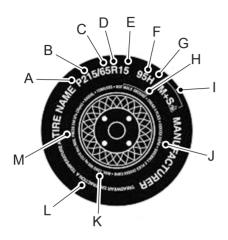
P215/65R15 95H is an example of a tire size, load index and speed rating. The definitions of these items are listed below. (Note that the tire size, load index and speed rating for your vehicle may be different from this example.)
