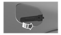
Insert the emergency opening tool in the position shown and gently pry the fuel door open.
