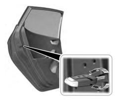
A child safety lock is on the rear edge of each rear door. You must switch the child safety lock separately on each door.
