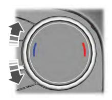
Turn the control on the left-hand side of the climate control to set the left-hand temperature.
