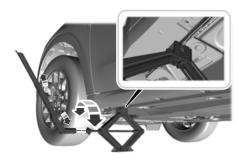
Remove the lug nuts with the lug wrench.
