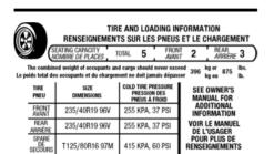
Payload is the combined weight of cargo and passengers that your vehicle is carrying. The maximum payload for your vehicle appears on the Tire and Loading label. The label is either on the B-pillar or the edge of the driver door. Vehicles exported outside the US and Canada may not have a tire and loading label. Look for "The combined weight of occupants and cargo should never exceed XXX kg or XXX lb" for maximum payload. The payload listed on the Tire and Loading Information label
