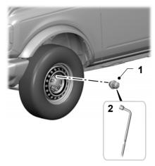
8. When you are changing a flat front tire, connect the extension block to the jack loadrest using the wing bolt as shown. Connect the jack handle to the jack, and use the lug nut wrench to operate the jack.
