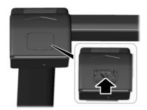
**Note:** The rear crossbar is part of the clamping system. If you removed the crossbar you must install it first for proper attachment to the hard top.
