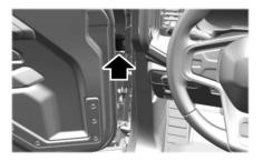
10. Remove the upper hinge bolt. **Note:** Store the hinge bolts in the pocket of the tool pouch.
