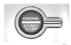
2. Press the push button ignition switch. **Note:** The engine may continue cranking for up to 15 seconds or until it starts.
