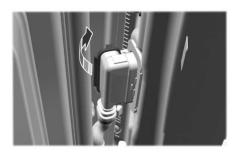
To release the door harness connector, open the connector door. Pull the connector straight out.
