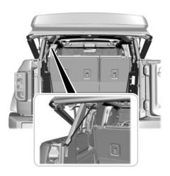
3. Lift the rear of the soft top and support it with the soft top strut.
