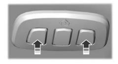
Press and hold the outer two function buttons simultaneously for approximately 10 seconds until the indicator light above the buttons flashes rapidly.
