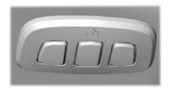
The universal garage door opener replaces the common hand-held garage door opener with a three-button transmitter integrated into the driver's sun visor.
