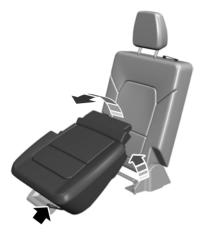
Pull the strap at the front of the seat cushion. Then, flip the seat cushion up to the vertical position.
