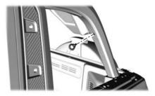
Install the eyebolts located in the Ford onboard storage kit into the rear cargo area pillars.
