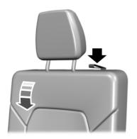
2. Pull the strap on the top of the seat backrest to fold it forward.
