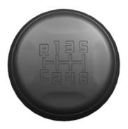
When shifting into crawler (C), make sure your vehicle is completely stationary and that the engine speed is below 1500 RPM.
