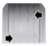
When the tread is worn down to one sixteenth of an inch (2 mm), tires must be replaced to help prevent your vehicle from skidding and hydroplaning. Built-in treadwear indicators, or wear bars, which look like narrow strips of smooth rubber across the tread will appear on the tire when the tread is worn down to one sixteenth of an inch (2 mm).
