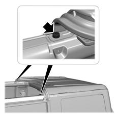
Remove the two fasteners that secure the rear roof panel at the C-pillar using the provided head driver and ratchet.
