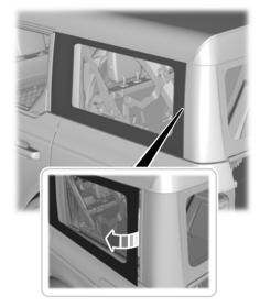
1. Release the rear edge of the panel by pulling the fabric out of the slot.
