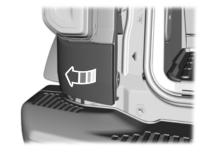
Remove the lower trim piece by disengaging the retaining tabs. Pull from the inside edge first, then pull from the outside edge.
