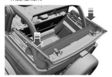
Press down on the driver side and passenger side of the soft top to fully secure it.  To return to the partially open position, press down and lift the handle on the driver side of your vehicle to unlatch the soft top, then rotate the soft top forward.
