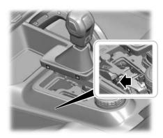
Insert a screwdriver between the shifter boot material and trim ring to access the retainer tabs from the top panel trim ring.
