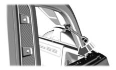
2. Use the ratchet tool provided in the kit to assist in tightening the eyebolts. The eyebolts should rest in the groove of the handle. Using the tool as a lever, apply force until fully tightened.
