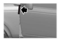
Locate the fender protector in the tool pouch and install it over the fender edge near the top door hinge.
