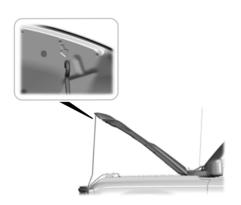
3. Open the hood and support it with the hood strut.
