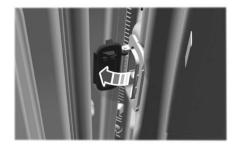
Insert the door harness into the connector.
