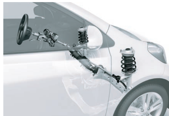
2 A newly developed centre take-off steering gear
