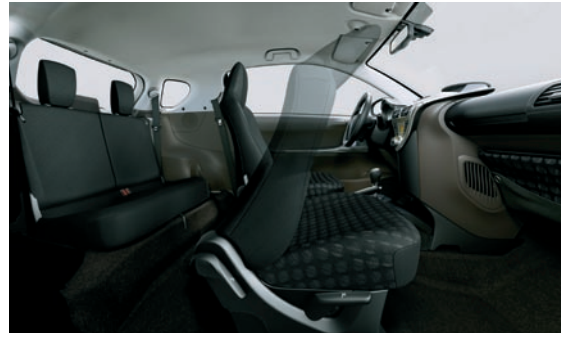
4 Newly developed slim-backed seats provide 40 mm more knee room for rear seat passengers.
