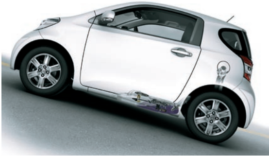
3 A super flat under-floor fuel tank, only 120 mm in depth
