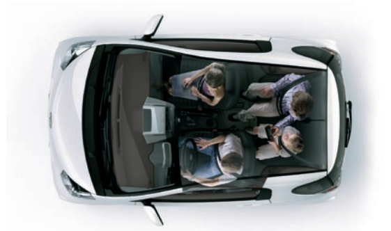
6 An asymmetric dashboard design allowing a significant increase in leg room for the front passenger
