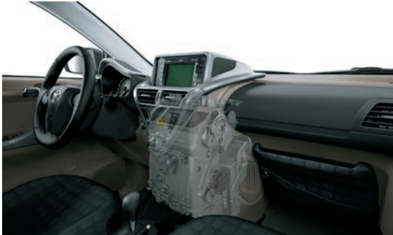
5 An ultra-compact air conditioning and heating unit, 20% smaller than a conventional unit without sacrificing performance
