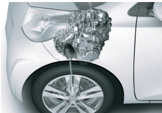
1 A uniquely developed front-mounted differential integrated in a conventional transmission layout
