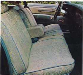
Newport optional 50/50 Willamberg cloth bench seat with vinyl accents, and dual folding center armrests, with passenger-side recliner on 4-door models.
