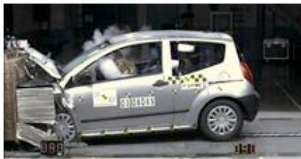
Offset crash test at 64km/h
